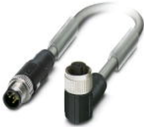
Bus system cable, CANopen®, 5-position, PUR halogen-free, Gray RAL 7001, shielded, Plug straight M12-SPEEDCON, A-coded, on Socket angled M12-SPEEDCON, A-coded, Cable length: 1 m
