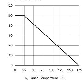
TOTAL POWER DISSIPATION vs. CASE TEMPERATURE
